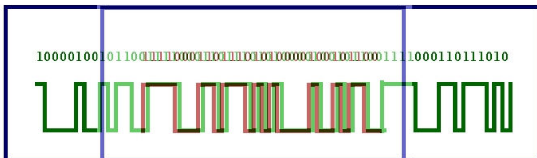
Partial Correlation of Identical Receiver and Satellite PRN Codes
